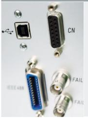
Every generator is equipped with both GPIB and USB interfaces for remote control. Fail1 and Fail2 inputs are implemented for DUT monitoring purposes.
